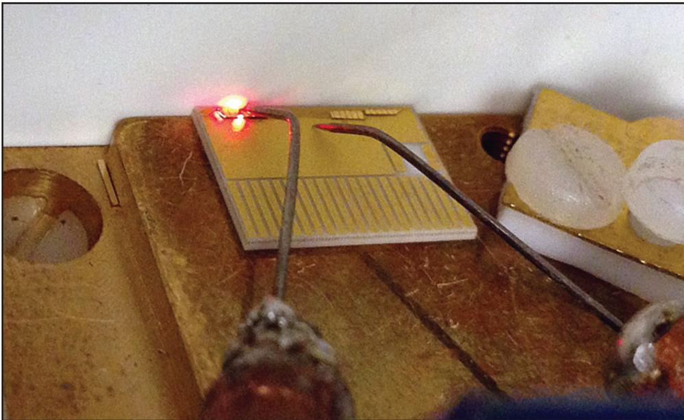
The first demonstration of an InGaP/InAlGaP-based orange laser emitting at 608 nm has been reported by researchers in Saudi Arabia. Using a cost effective approach, the work is aimed at filling a wavelength gap in the visible spectrum for commercial semiconductor lasers, enabling a wide range of uses including lighting and VLC.
